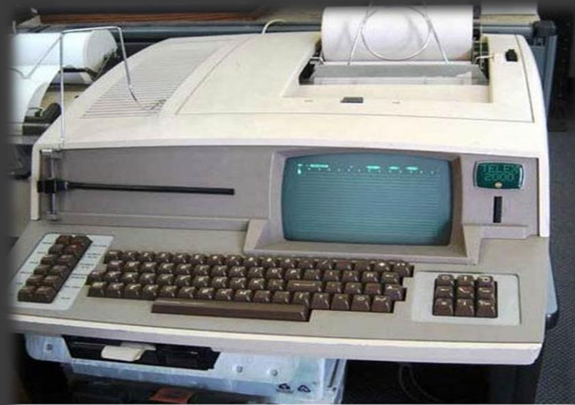
The Sagem Teleprinter 2000. Early 1980's. This machine introduced the VDU screen and the 5 inch floppy disc as the storage medium.
